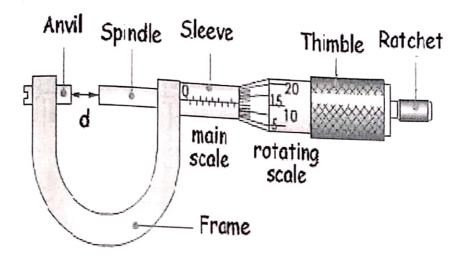
For example for a screw gauge with a pitch of 1mm and 100 divisions on the circular scale. The least count is = 1 mm/100 = 0.01 mm
